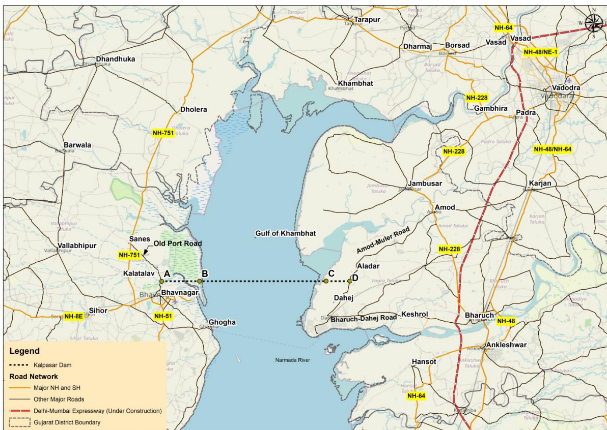
Figure 2.25: Alignment of Kalpasar dyke and access roads
